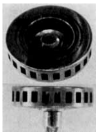
Fig. 1.—Centrifugal wheel atomizer. Wheel has radius = 2.50 cm., 24 vanes, vane height = 5.82 mm., width of vane opening = 3.51 mm.
